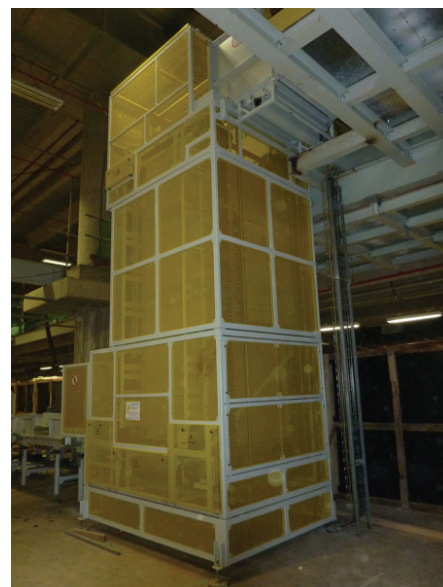
Photo: a typical NERAK Continuous Vertical Conveyor Type S316Gep installed in a modern BHS
